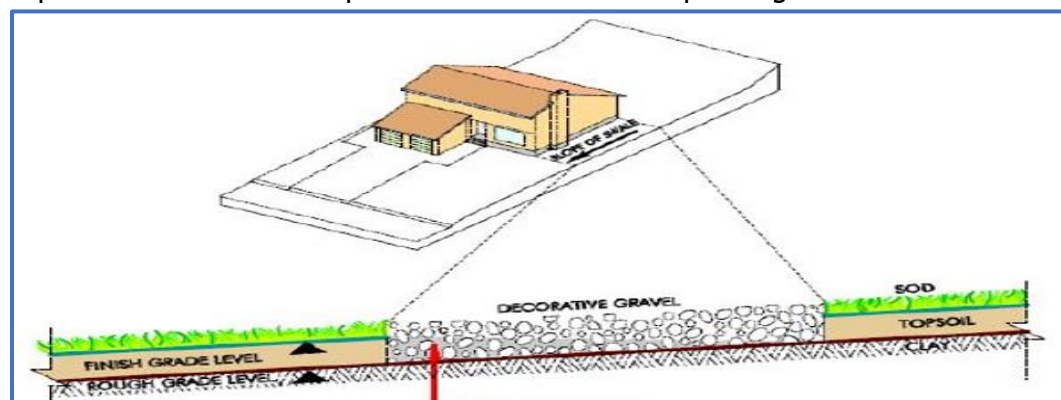
Installing decorative material on RG surface creates ponding
