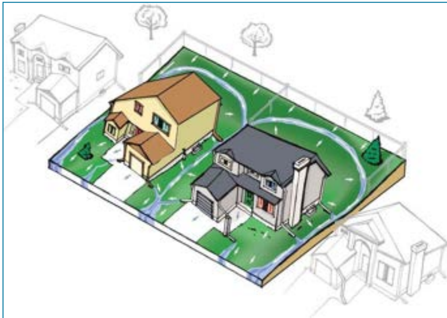
Example of "Back to Front" Lot Drainage
